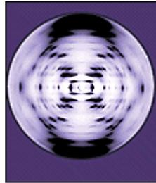
*The X ray diffraction pattern produced by crystallized DNA. The dimensions of the double helix can be calculated from the positions of the black regions.*
