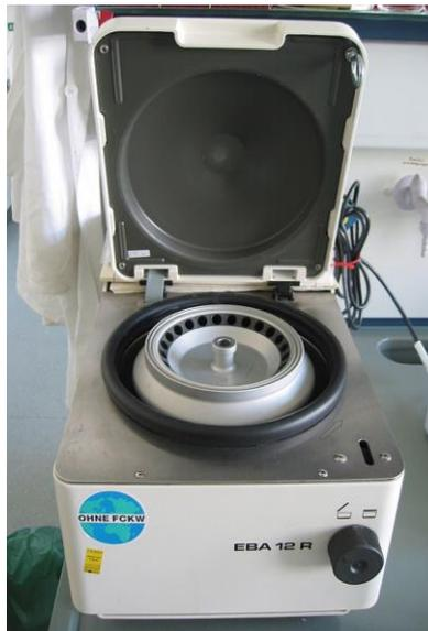
*A centrifuge. The centrifuge tubes are placed in the holes around the rim of the central part, which spins fast when the lid is closed.*
