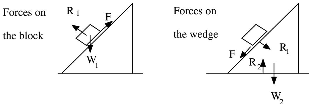
Since the block is trying to slide down the wedge,  $F$  will act upwards on it, and there will then be an equal and opposite force  $F$  acting downwards along the slope of the wedge.
